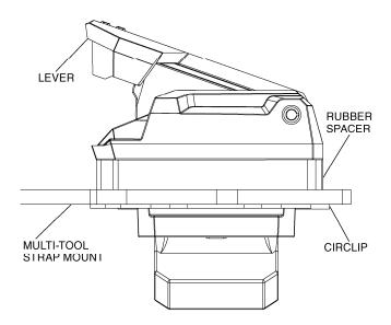
3. Make sure the Pro-Connect<sup>™</sup> latch lever are in the open position then locate the multi-tool strap mount onto the vehicle bed (or compatible accessory) by aligning each Pro-Connect<sup>™</sup> latch with his corresponding bed installation hole. Lock the multi-tool strap mount in place by pressing down the two Pro-Connect<sup>™</sup> latch levers.
