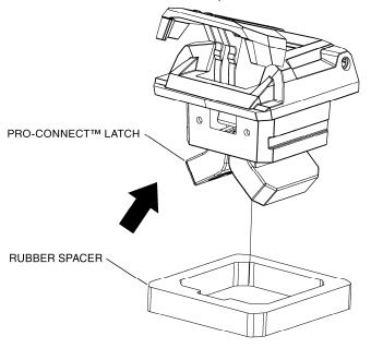
2. Insert the Pro-Connect™ latch in the multi-tool strap mount installation holes and secure them using the circlips.
